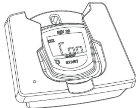
Underneath the display panel there is a key marked "Start". Different equipment functions can be initiated with this key.
